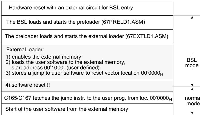
Figure 7: Action items how to load user software to the external memory and leave the BSL mode
