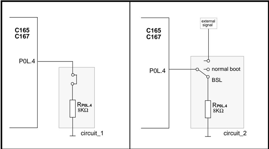
Figure 2: Two exemplary circuit diagrams for BSL entry via plug or switchable circuit
