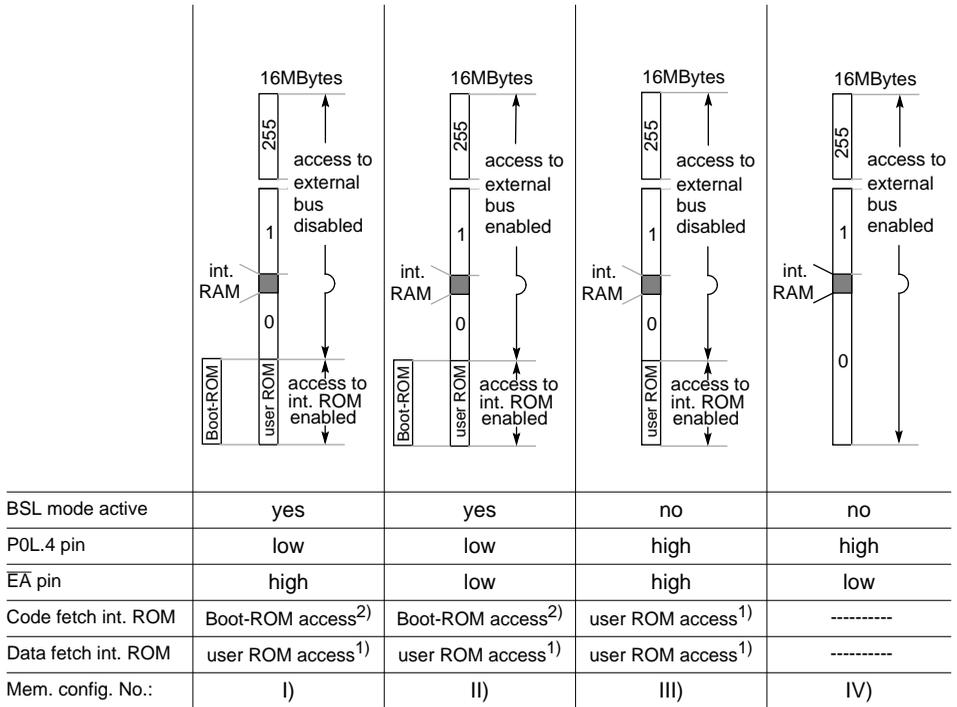
1) All accesses to the internal address space (00'0000<sub>H</sub> - 00'7FFF<sub>H</sub>) of a ROMless version of the C165/C167 result in undefined read values
