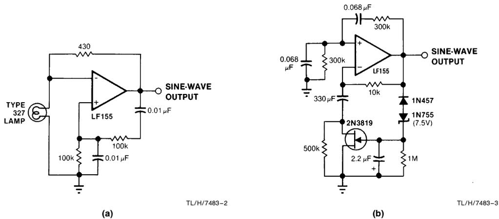
**FIGURE 2. A basic Wein bridge design (a) employs a lamp's positive temperature coefficient to achieve amplitude stability. A more complex version (b) provides the same feature with the additional advantage of loop time-constant control.**
