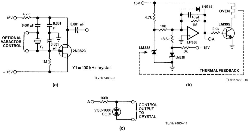
**FIGURE 7.** Stable quartz-crystal oscillators can operate with a single active device (a). You can achieve maximum frequency stability by mounting the oscillator in an oven and using a temperature-controlling circuit (b). A varactor network (c) can also accomplish crystal fine tuning. Here, the varactor replaces the oven and retunes the crystal by changing its load capacitances.
